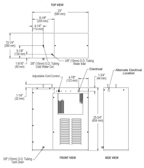
**NOTE:** It is important to insure proper ventilation. Allow a minimum clearance of 12" (305mm) in front and 3" (76mm) in the rear of unit.
